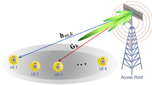
Fig. 1. Generalized AS approach to realize SWIPT architecture.
