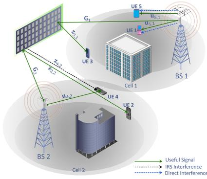
Fig. 1. An IRS-assisted multi-cell downlink network.
